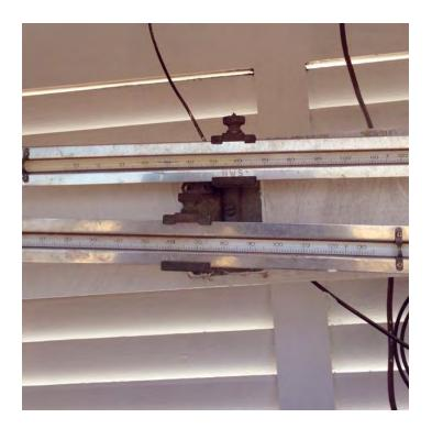
The traditional thermometers to monitor daily maximum & minimum temperature; housed in a doubled-louvered wooden box mounted at about 1.25 m high.
