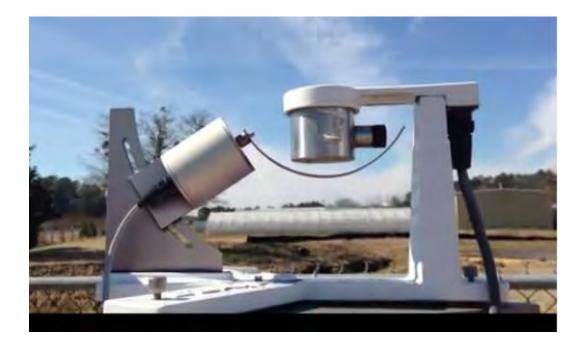
• Measures Sun's irradiance at 6 bands, 415, 500, 615, 673, 870 & 940 nm; measures total horizontal, diffuse & direct portion of the spectrum.
