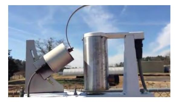
• This measures solar irradiance at 300, 305, 311, 317,325, 332. & 368 nm; used to estimate optical depth.
