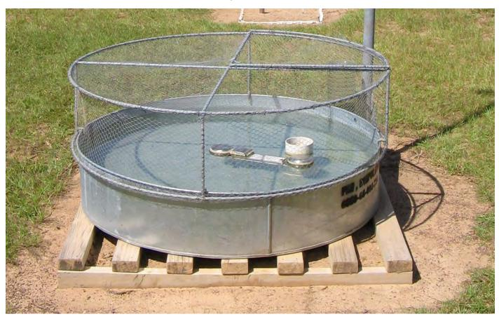
A cylinder or circular pan with 120.7 cm diameter, 25 cm in height is used to measure evapotranspiration; this provide guidance for irrigation of the crops.
