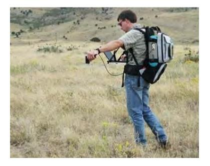
The FieldSpec portable spectroradiometer offers the modular Goetz spectrometer engine with a spectral range from 350 nm to 2500 nm
