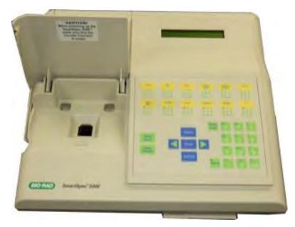
The UV/visible SmartSpec 3000 spectrophotomer has a working wavelength range of 200–800 nm.
