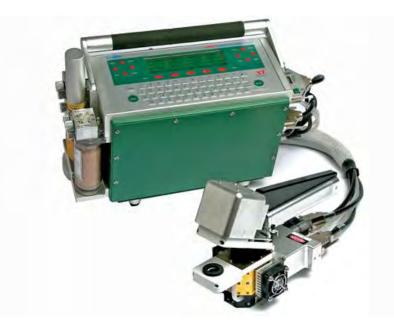
The LI-COR 6400 utilizes gas exchange principles to measure the photosynthesis rates of plants.
