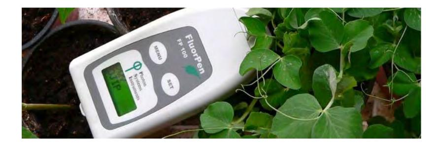
• FluorPen is a portable, battery-powered fluorometer that enables quick and precise measurement of chlorophyll fluorescence parameters in the laboratory, greenhouse, or in the field.
