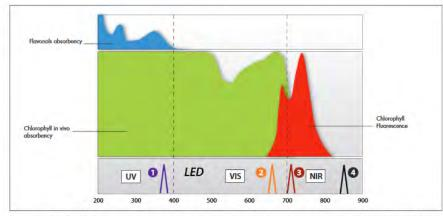
A wavelength in the UV **O** is compared to a second wavelength in the red **O**. Both wavelengths excite the fluorescence of chlorophyll, but only UV is affected by the presence of flavonols. By using these two wavelengths, the DUALEX<sup>®</sup> SCIENTIFIC calculates a numeric value directly correlated with chlorophyll content in the measured sample.
