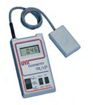
This digital UVX Radiometer is used with one of the three interchangeable sensors (ordered separately) for measuring 254nm, 365nm and 302nm UV wavelengths.
