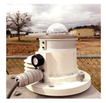
This gadget measures Sun's UV-B radiation from 280-320 nm; measured UV radiation is being used to project Harmful Sun's UV so that beach goers can apply the right kind of sunscreen lotions (SPF) to protect against cancer causing radiation.
