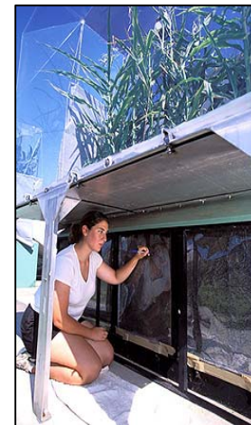
Mini-rhizotron system for non-destructive root growth and development
