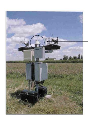
Broadband UV meters measure ultraviolet radiation in the UV-B spectral range of 280-330 nanometers.
